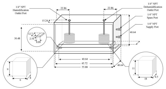
Fig.: Humidification/Dehumidification Unit
